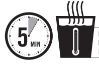
FOR PROPER INSTALLATION, SOAK AIR LINE TUBE ENDS IN HOT WATER BEFORE INSTALLING ONTO BARBED FITTINGS.
