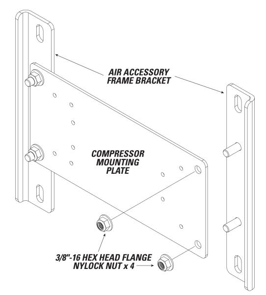
INSTALL THE AIR COMPRESSOR - USE FOR STANDARD DUTY AIR COMMAND KITS 2900 & 2910
