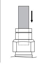
Gently pull on the air line tube to check for a secure fit.
