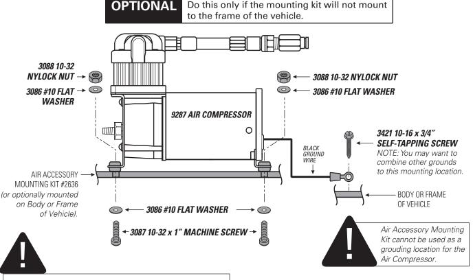
Mount to the drill holes made in the frame.
