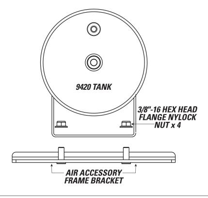
**1** Determine a location on the frame rail of the vehicle to mount the tank. This should be as close to the Air Compressor as possible.
