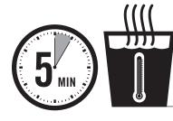
FOR PROPER INSTALLATION, SOAK AIR LINE TUBE ENDS IN HOT WATER BEFORE INSTALLING ONTO BARBED FITTINGS.
