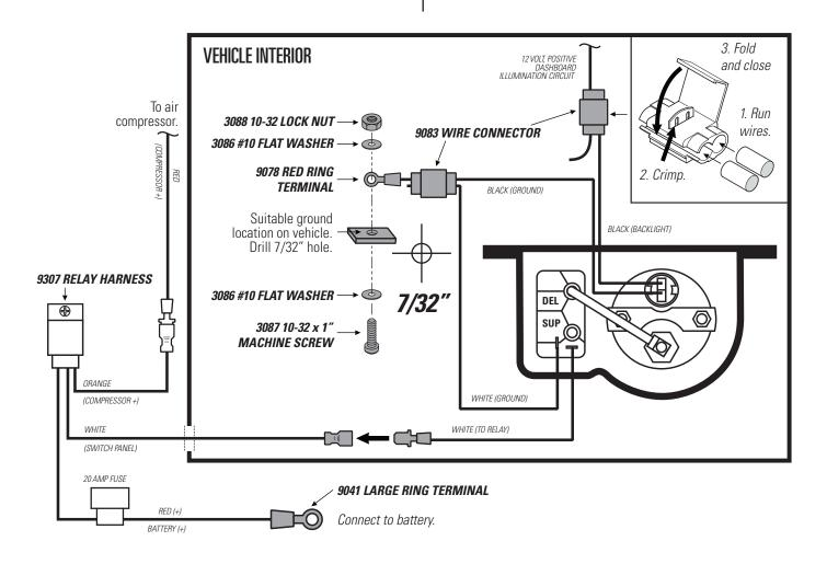
Install the Control Panel using the supplied fasteners.
