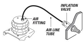
Place an air chuck onto the Inflation Valve and fill the system to **70 PSI**.
