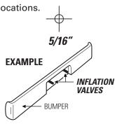
Install Inflation Valve assembly as shown.
