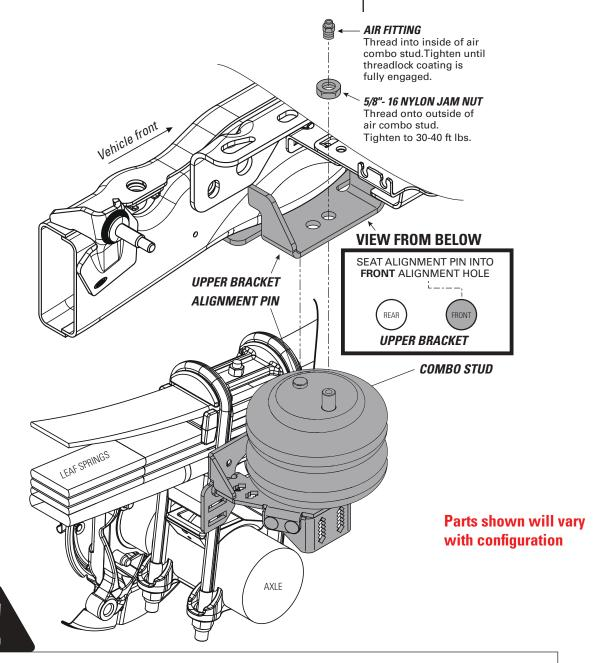
ALIGNMENT PIN ON AIR SPRINGS MUST BE INSTALLED TO FULLY SEAT INTO THE FRONT ALIGNMENT HOLE IN THE UPPER BRACKET. FAILURE TO DO SO WILL CAUSE IT TO BE PUSHED INTO THE BEAD PLATE, CREATING AN AIR LEAK, AND RESULTING IN AN AIR SPRING FAILURE THAT IS **NOT WARRANTABLE**.
