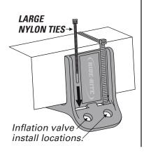
2 Select a protected location to install the inflation valves, such as the bumper or the body of the vehicle.
