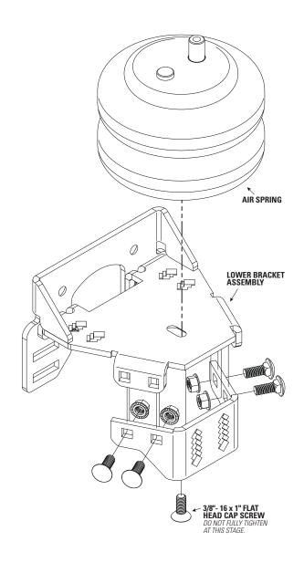
Fasten the air spring to the lower spring bracket. **DO NOT FULLY TIGHTEN AT THIS STAGE**.
