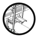
Fasten the air spring to the lower spring bracket. **DO NOT FULLY TIGHTEN AT THIS STAGE**.
