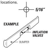
Install inflation valve assembly as shown.
